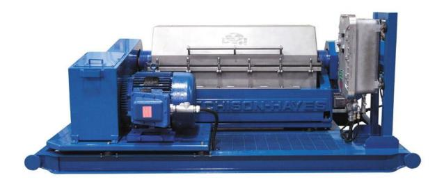
The HH 1448 Standard is a configuration of a drive system for a Decanting centrifuge. This configuration is the most basic of many available configurations. The Centrifuge bowl is driven by a main drive motor and the conveyor is driven through a planetary gear box with a simple torque arm setup.
